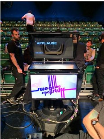
**16 x9 Talent Monitor/TV.** We offer consumer TV's with VESA plate attachment rigging and SDI input options using adapters. We can supply pretty much any size with 24" as standard but have also rigged two 32" as one system
